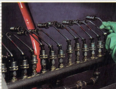
Strict cleanliness specifications are achieved through the use of pressurized oil flushing machines.
